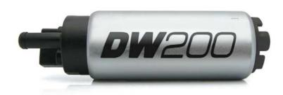
The DW200 flows 255lph at 40psi and is a popular choice for many high performance applications which can be fitted with a standard fitment pump. The DW200 features a quiet and reliable turbine impeller which is compatible with pulse width modulated pump drivers. The pump also features an encapsulated armature for compatability with ethanol based fuels. All DW fuel pumps are backed by a 3-yr no fault warranty.
